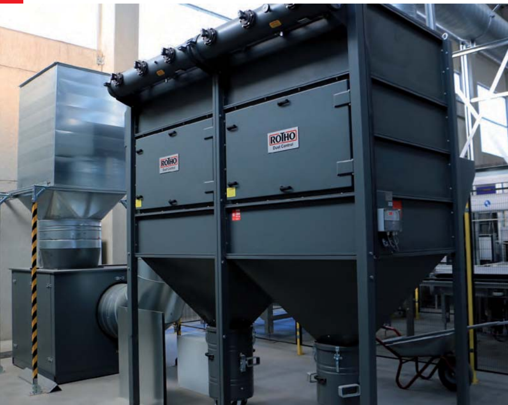
Filter system with automatic dust cleaning device
